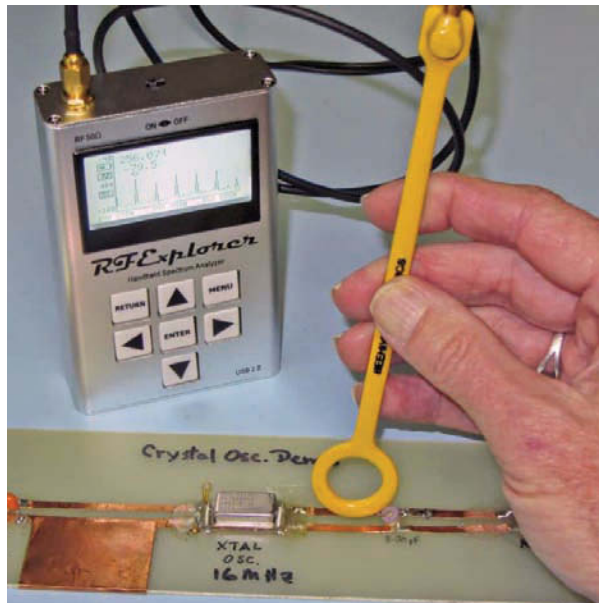
Probing a crystal oscillator demo board with the RF Explorer displays usable harmonics.
