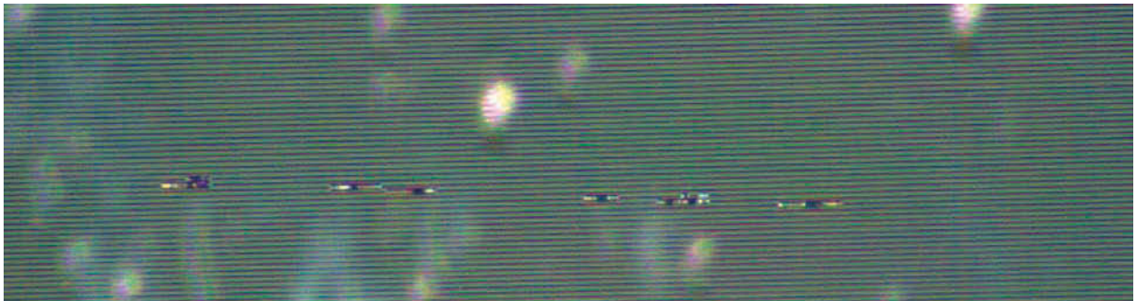
FIGURE 1. An optical image shows damaged conductors in an LCD.
